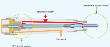
In modern heavy duty diesel engines, traditional detergents at treat rates required to have any impact, are simply not practical, as a means to prevent injector fouling. At the same time, the need to remove deposits in and around the injector valve seat and nozzle has become even more critical to overall performance.
