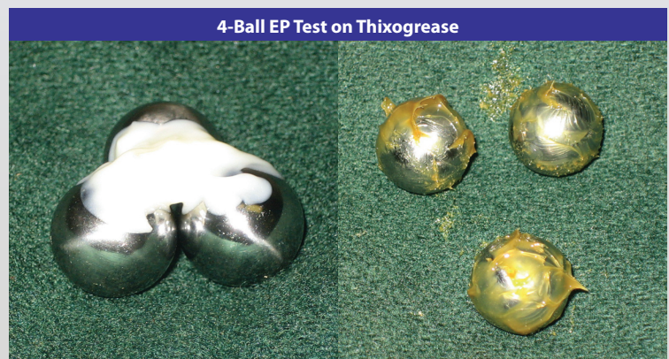
Picture 2: Steel balls coated in Thixogrease remain unmarked and moving freely in 4 ball EP wear test with 4 times the load of the previous test.
